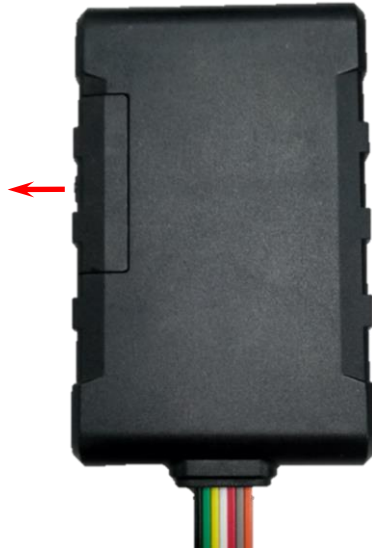
Figure 10. Open the SIM card cover
